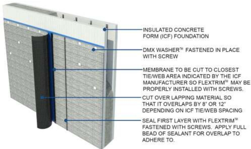
Figure 18 Vertical Joining on ICF
