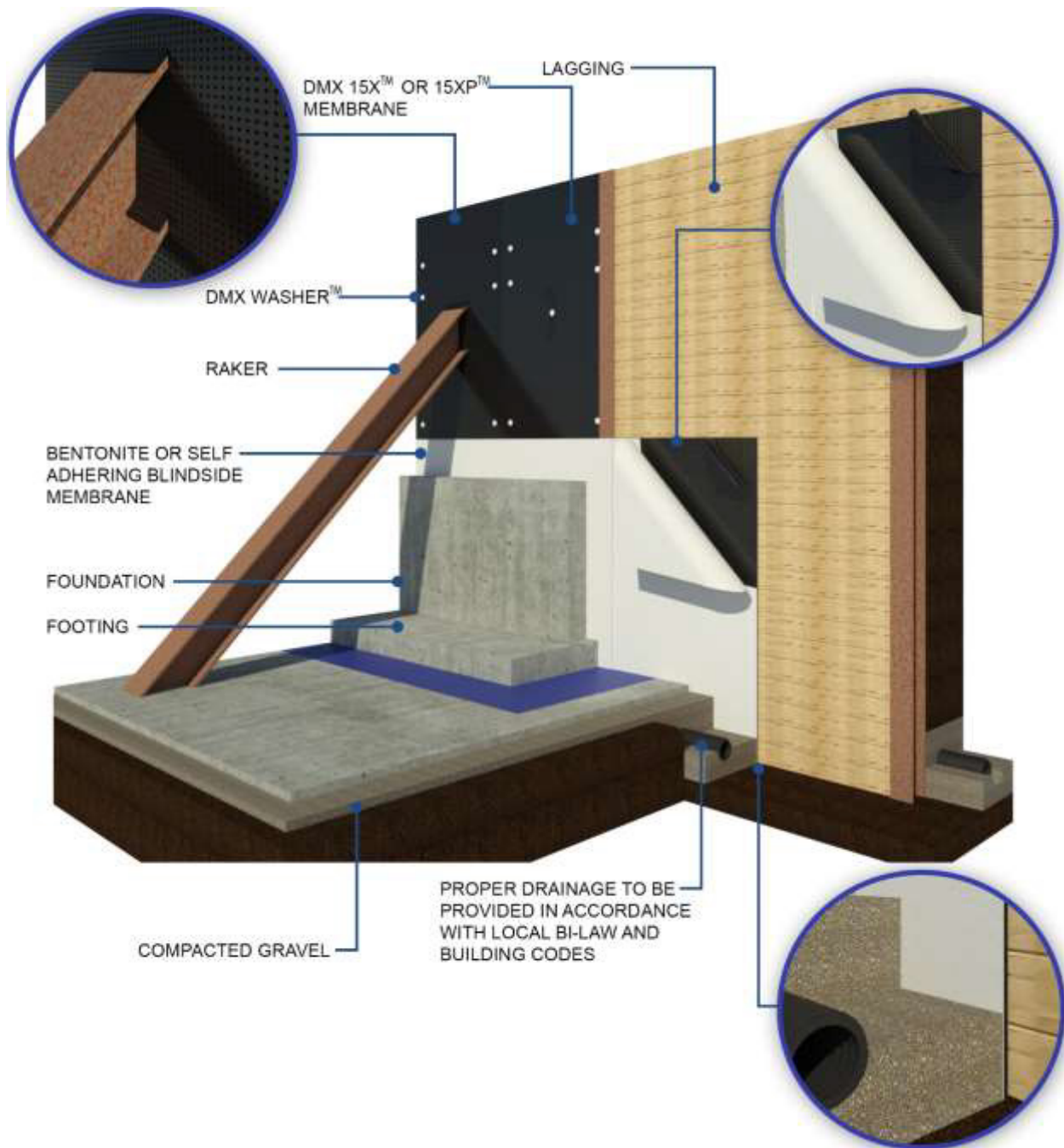
Figure 2 DMX Drain 15X in Blindsided Waterproofing Assembly
