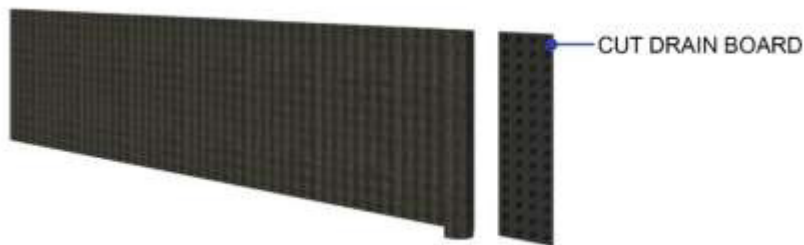
Figure 12 Sealing End of Roll without FlexTrim Step 2
