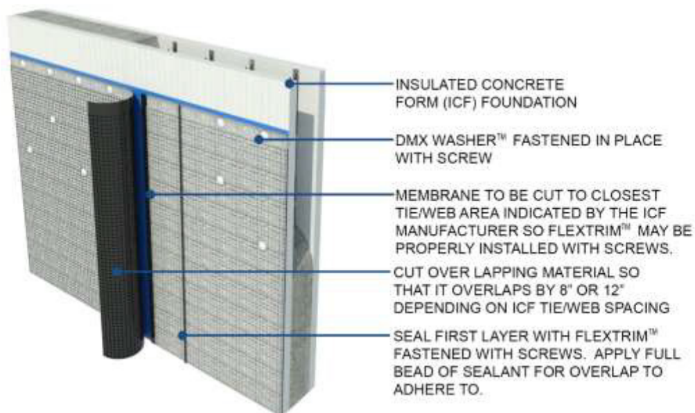
Figure 18 Vertical Joining on ICF
